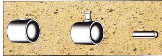
Tracer Wire, Marker Magnet, and Metallic Pipe
