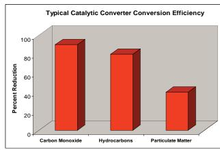
Bobcat Exhaust Purifiers represent the most advanced catalyst technology designed for high reductions of diesel soot, carbon monoxide and hydrocarbons. Each exhaust purifier contains a brazed steel catalyst honeycomb, the highest quality catalyst substrate in the industry.
